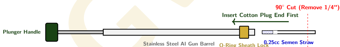
Fig 3: Proper AI Gun Assembly & Straw Insertion
